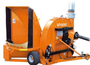
The reducer gearbox on the V59 HV lowers the input speed from 1000 RPM at the PTO to 650 RPM at the rotor. With a discharge velocity of 118 MPH (189 km/h), this 8-paddle rotor makes the V59 HV the largest volume displacement blower on the market.
