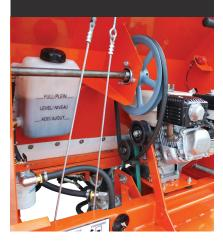
The drive wheels are directly driven by two hydraulic motors fed by a sturdy hydrostatic pump, thus eliminating the need for costly and complicated maintenance of a differential or gear box.
