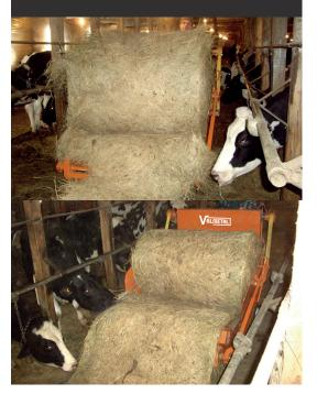
Automatic tensioners always provide constant tension on the two chains of the apron. The round bale unroller is driven by a 9 Hp Honda Motor and a high performance hydrostatic pump.
