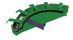
▲ The heavy-duty design of Badger's reverse curve provides ease of operation and longer life. The curve's full bottom features 3/16" steel plate reducing gutter bottom wear and allows smooth, steady chain flow.
