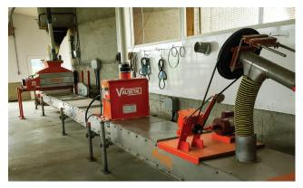
THE ENTIRE CONVEYOR STRUCTURE IS MADE OF Stainless steel to resist corrosion and Abrasion
