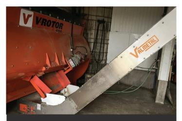
**REGULATING THE FLOW** This type of conveyor is ideal for regulating the flow from the mixer directly to belt conveyors and feeders.
