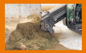
Hay knife kit allows direct loading of hay
